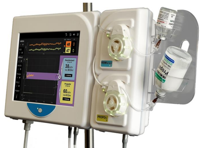
Fig. 12 – AutoTIVA (model AT-901) closed-loop TIVA delivery system. Advanced prototype and research platform (not for sale).
